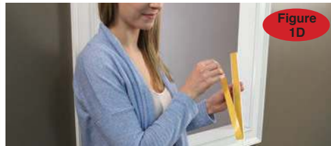
1D Peel off double sided adhesive from behind the Miracle Fit Base.
